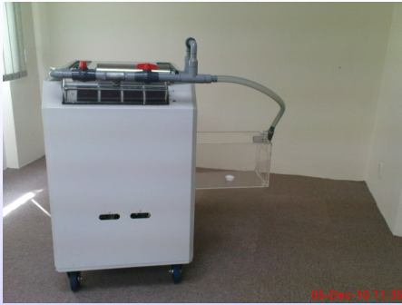
Sterilizing Chamber enclosure was constructed to facilitate the lab test
