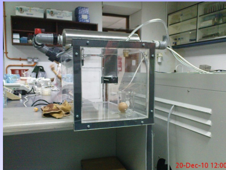
Inoculated eggs were placed inside the sterilizing chamber for test
